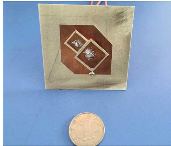
Fig. 2-4 Processed Antenna
