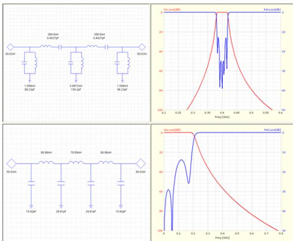
Fig. 5. Filters for the RF ports.
