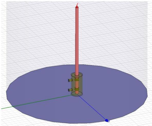
Fig. 3. Approximate HFSS model of plasma antenna.
