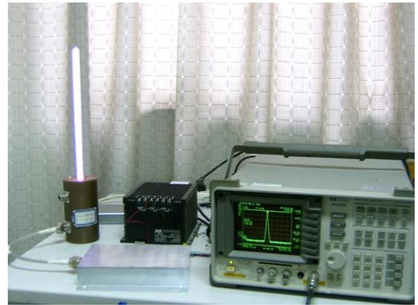
Fig. 1. Ionized plasma antenna prototype.
