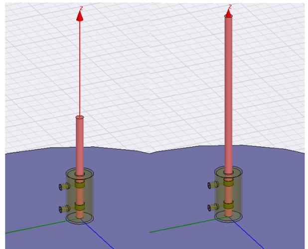
Fig. 6. Reconfigurable length of plasma antenna.
