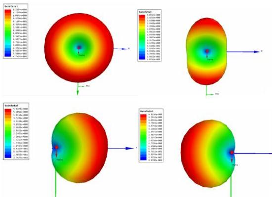
Fig. 9. Two elements plasma antenna array pattern at 300MHz.
