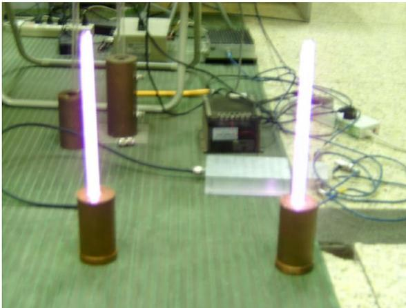
Fig. 8. Two elements plasma antenna array.
