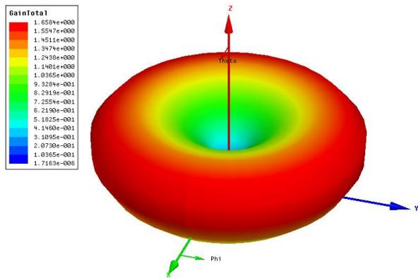
Fig. 4. Radiation pattern of plasma antenna 3D model.
