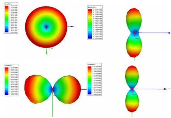
Fig. 10. Two elements plasma antenna array pattern at 600MHz.
