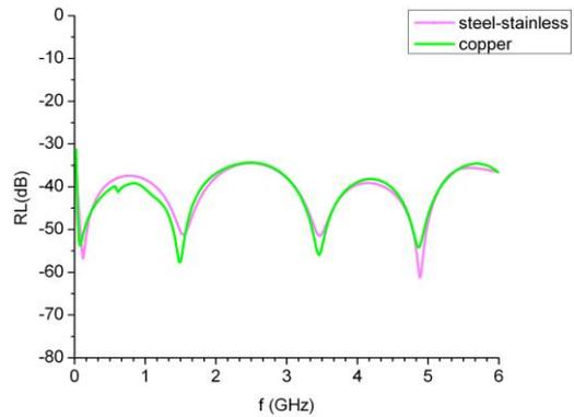
d) RL comparison for steel-stainless and copper
