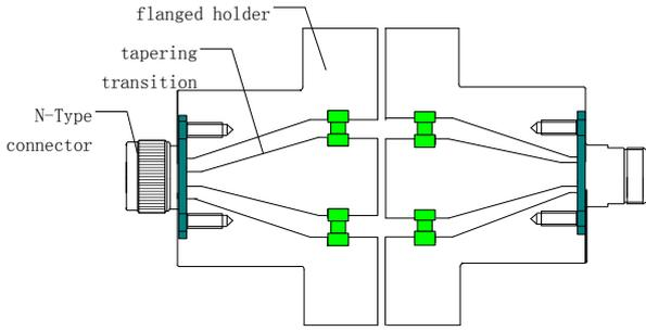
Fig. 1. The sketch of novel flanged coaxial tester
