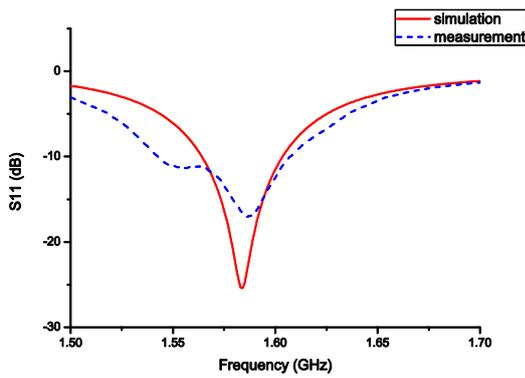
Fig. 3. Simulated and measured reflection coefficients of the proposed GPS antenna.
