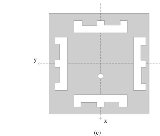
Fig. 1. Geometry of the single-feed circularly polarized antenna for GPS: (a) top view, (b) cross-sectional view, and (c) bottom view.
