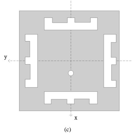
Fig. 1. Geometry of the single-feed circularly polarized antenna for GPS: (a) top view, (b) cross-sectional view, and (c) bottom view.
