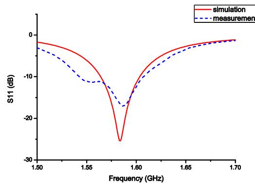
Fig. 3. Simulated and measured reflection coefficients of the proposed GPS antenna.
