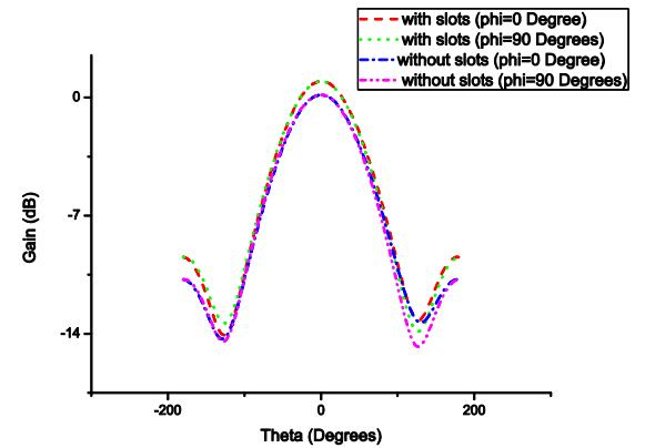
Fig. 5. Comparison of antenna gain with/without the four E-shaped slots at the frequency of 1.57542GHz.
