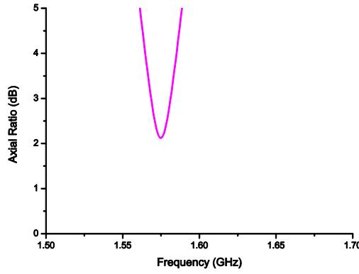
Fig. 4. Axial ratio of the proposed antenna.
