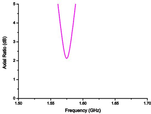
Fig. 4. Axial ratio of the proposed antenna.
