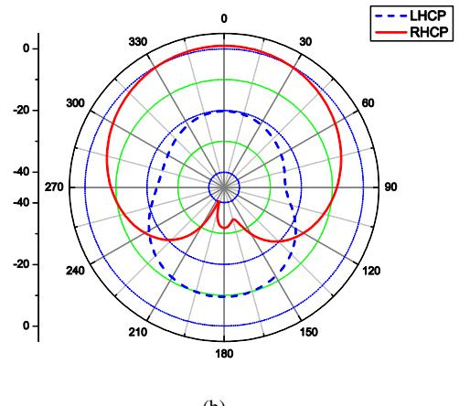
Fig. 6. Normalized radiation patterns of the proposed antenna at 1.57542GHz: (a) xz-plane and (b) yz-plane.
